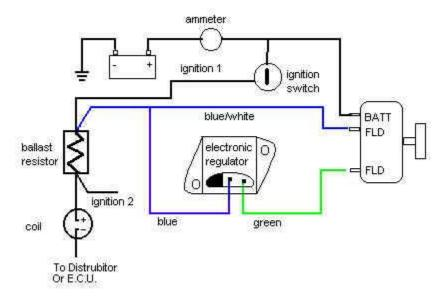
With the above diagram, you can upgrade your charging system from the 30 to 46 amp alternator to a 60 amp alternator.
