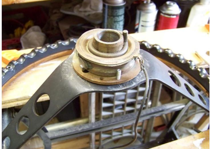
... it was welded in place. If you don't have a welder, or don't trust your welding skills, have a professional do this. The consequences of a failed weld here could be devastating.
