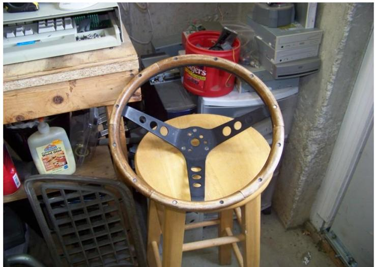
Using the horn ring as a guide, I centered it, marked and drilled holes so the bolts that mount the ring and horn button can pass through the wheel and mount the hub that I will use from a un-restorable original.
