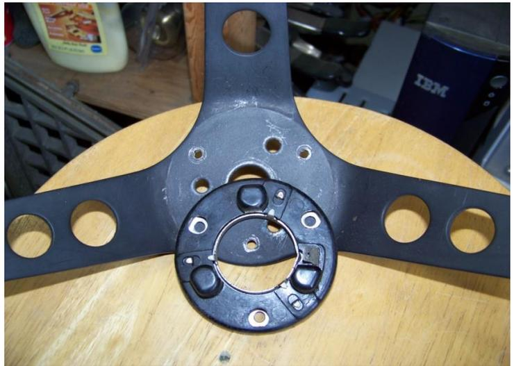
Here is the old steering wheel where I cut off the hub to use for the new wheel.
