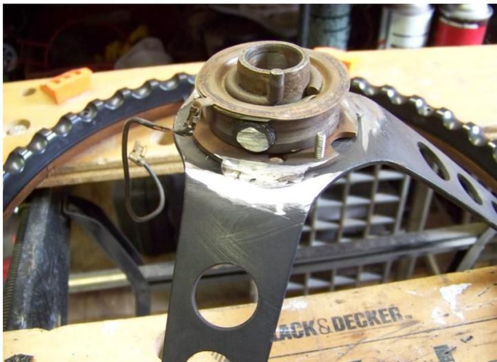
The original mounting bolts were too short after passing through the new wheel, so longer bolts were needed.
