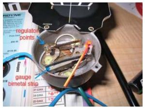
was due to a bow in the bimetallic arm that you can see clearly in the picture. I gently persuaded it to start out straight, which moved the needle to just below the "E".
