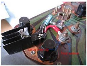
resistance. If your needle only goes half or three quarters, you have more work to do because the smallest resistance your tank sender is going to give is about 10 ohms (when full). Now connect the temp gauge "S" to the chassis. Your temp gauge should act the same way. If both gauges are not working at this point, verify that you have 12V at the input and 5V at the output. If all is well, reinstall the instrument panel. You're done.
