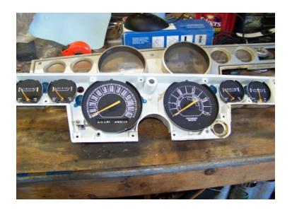
Next is to remove all the gauges. TIP: the Performance Indicator comes out the back while all the others come out the front.
