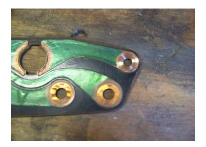
Clean the pins carefully. The ones on the large board are tight and in good shape but if they are lose they can be repaired.
