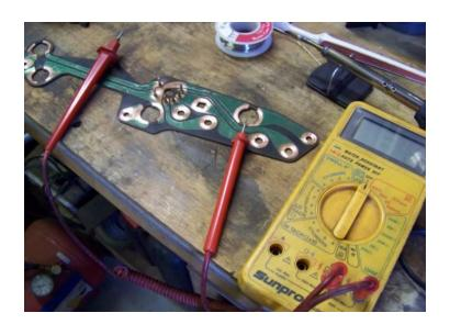
You can see here on the small board that the pins are loose and ready to fall off.
