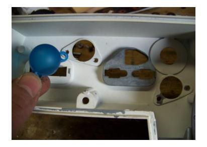
Here is the end of the large board and you can see the dark copper color on the contacts. Get out some steel wool and clean these up.
