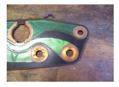
Fresh clean contacts! Do this for all the exposed board mounting points, the gauge contact points and the cresent contacts for the bulb sockets.
