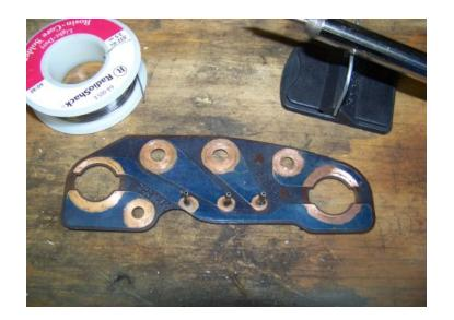
Here two of the three pins are soldered. Once they are done they will be tight and have the proper contact needed to keep the juice flowing to the lights and gauges.
