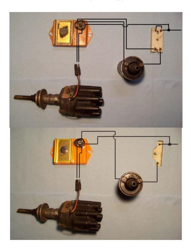
With the above diagrams, you can upgrade your ignition system from points to electronic with original Mopar components. Choose which type ECU/ Ballast you want to use then gather the parts (distrubitor, harness, ECU) from a swap meet or salvage yard. Remember the ECU needs to be grounded and the wiring colors need to be checked as the donor vehicle and your car may be different. Thats why wire color was omitted from the diargams.
