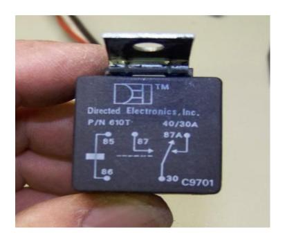
If you're not up on your relays this is the diagram on how they work. pole 86 is grounded and when power is put to pole 85 it activates an electromagnet pulling the internal switch from 87A to 87. When the relay is un powered, a connection is made from pole 30 to 87A. When energized the connection is switched to create a connection from pole 30 to pole 87.
