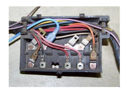
Now since you are pulling ignition on power before the fuse, you will need to add in an inline fuse connector to protect the circuit.
