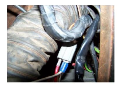
You can buy a buzzer or chime from your local auto parts store or electronics supply house. Just ground the chime and connect the power lead to the 87A pole on the relay.
