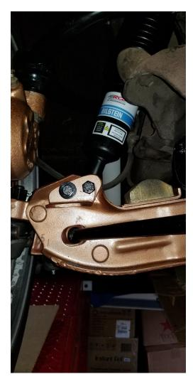
The pic on the left is the passenger-side bracket installed, and the pic on the right has the end-link installed but before there is any load on the suspension..
