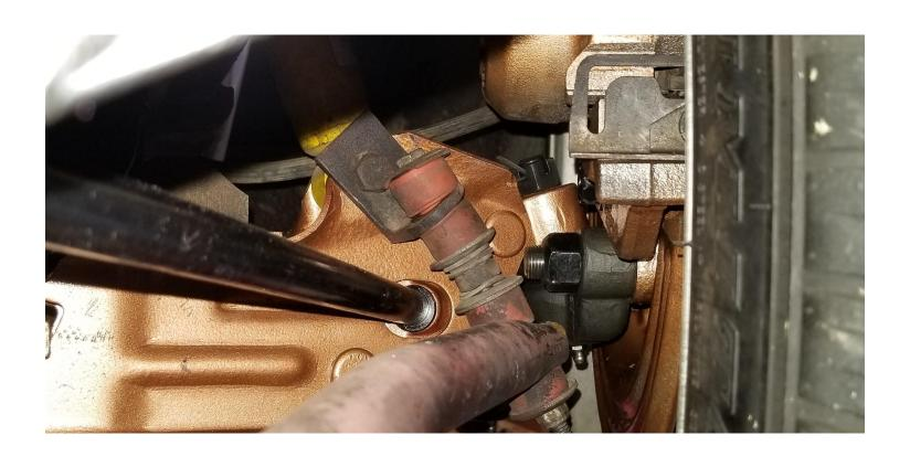
I decided to make my own. I started with making a template out of cardboard, and then transferred the shape to a piece of 2" x 2" angle steel from the local box store. The smaller hole gives the mount more stability for both deflection and up/down movement, and requires drilling a corresponding hole in the LCA. The largest hole is for the sway bar end-link, and the medium size hole is for the shock mount bolt.
