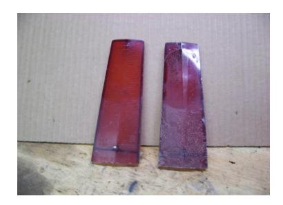
We are going to switch gears here. The other parts we worked with are of a hard plastic. The dome light lenses are much softer and is why they look so bad. They get stained and become opaque. Polish will not work here.
