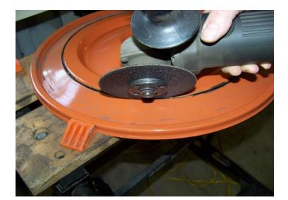
Same for the base. I used the crease in the base at the edge of where the filter sits to guide the grinder. The edges are cleaned up on the bench grinder.
