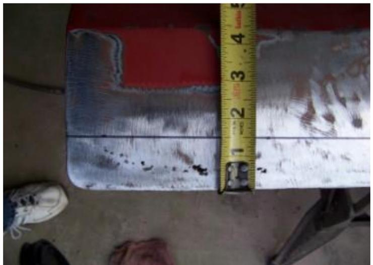
Using my 4 1/2 inch angle grinder with a cutting disc I carefully cut through the outer sheet metal along the marked line. Be careful not to cut too deep on the edges.
