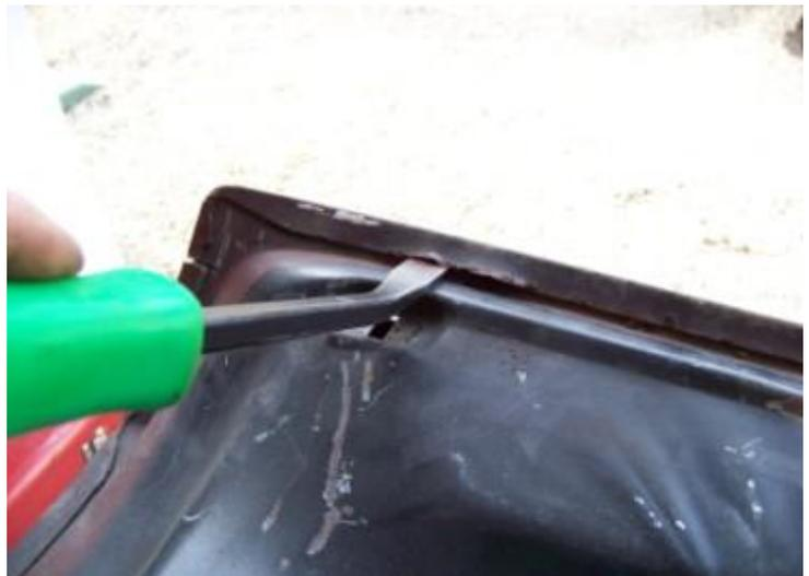
**When it looks like this stop and address the spot welds. You can see the sections that are still stuck and need work.**
