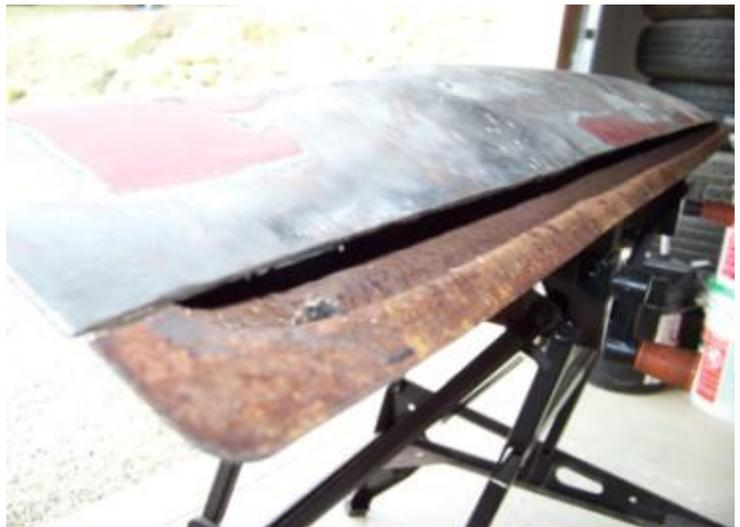
**I took the extra step of treating the bare rust with a spray rust converter. I did both sides of the inner lip and I sprayed as far inside the trunk as I could. Wait until it's dry and add a second coat. You do not want to do this repair again and now is the time to protect the metal. Other treatments like Por15 can be used as well.**
