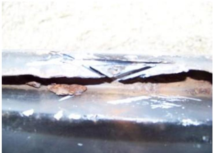
**...Then carefully grind the edge until you break through and can see the two separate parts. This will make it easier to pry the lip up around the welds.**
