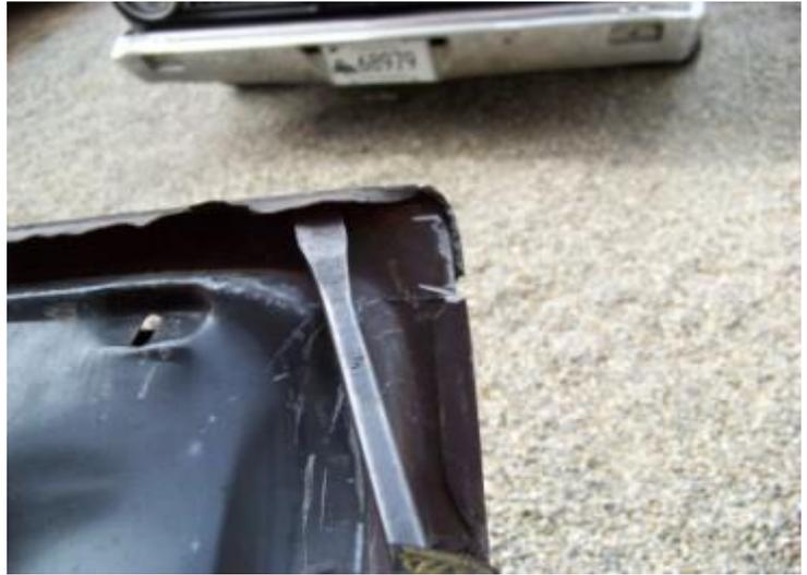
**And the lip is off. Don't toss the lip yet. We will need it as a template for the new sheet metal. Take this time to grind off any left over metal around the spot welds and clean up both sides of the inner lip with a wire wheel.**
