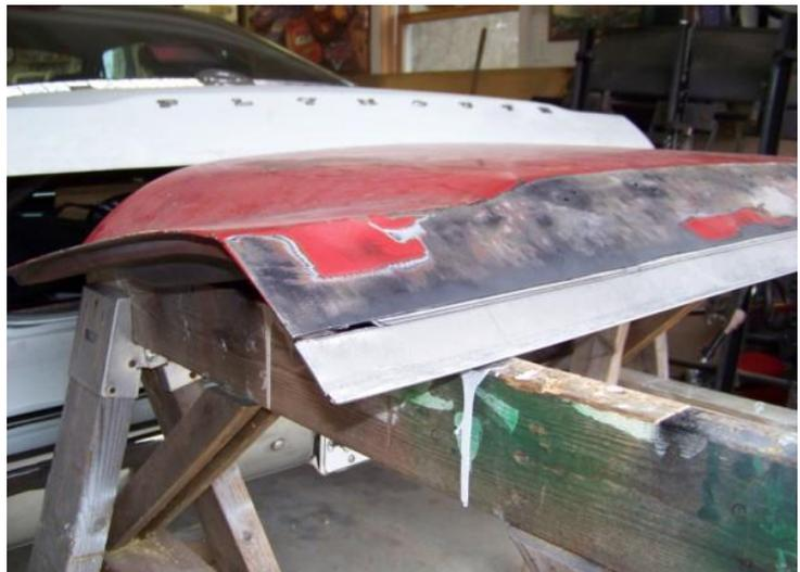
**You can see how I cut the ends to fit under the existing trunk metal. I'll need to do a little extra welding to close the gap here. The corners will need to be welded and ground to get the radius correct. That won't be too difficult.**
