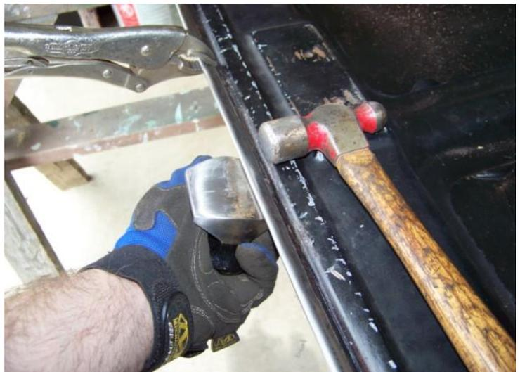
Once you get it close to closed, push one of the ends in tight to the trunk lip, clamp it down and continue to hammer and dolly the edge flatter and flatter.
