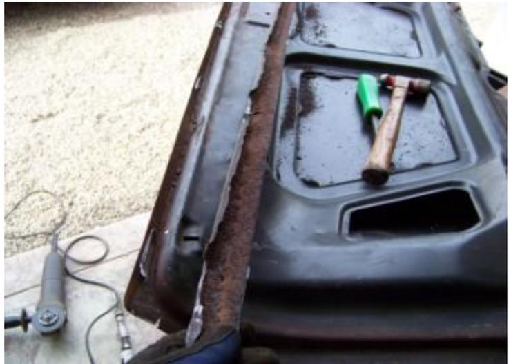
**Clean up the sheet metal with a file to remove any loose metal. Now would be a good time to blow out any debris or rust floating around inside the lid.**
