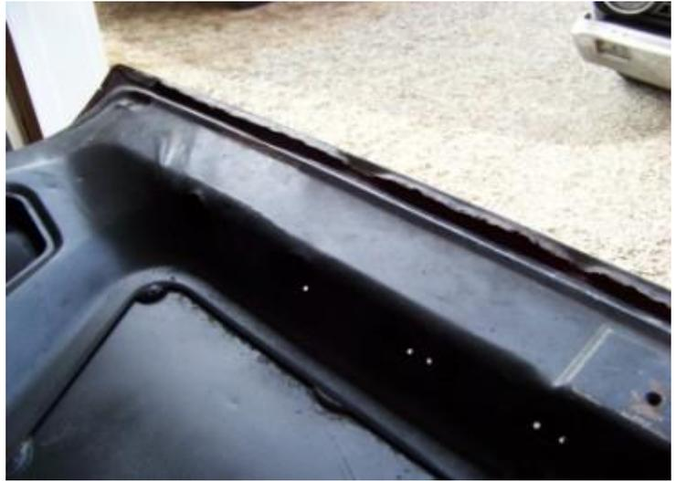
**Using the grinder cut around the weld like this to relieve the stress on the lip...**
