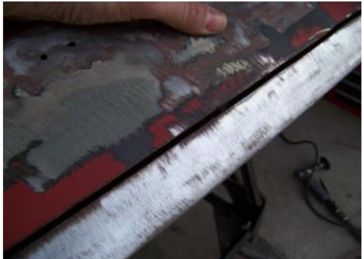
Using a small pry bar start to pry the inner lip up and away. Take your time and do not force it. There are spot welds that will need attention and we do not want to damage the inner trunk lid.
