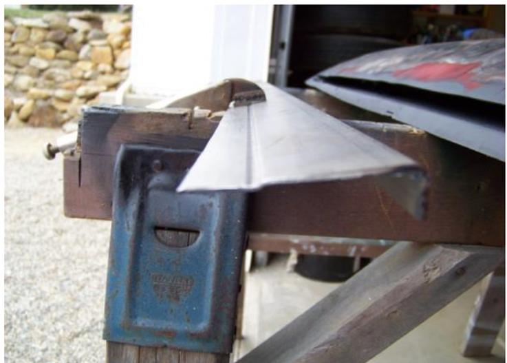
**You can cut the patch to fit to the cut edge and weld it that way, but I prefer to flange the metal. The flange pliers can be bought from Eastwood, but as always, I made mine.**
