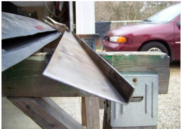
**I started by putting a flange on the top edge of the new patch so it fits under the the existing sheet metal on the trunk. This will allow us to weld the seam without blowing through and making the final body work a little easier for the novice.**
