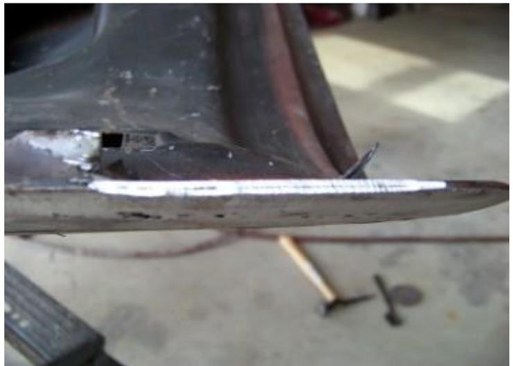
**Take the grinder and grind the inside lip off the corners. Now using the pry bar and a hammer, tap the lip off the trunk lid. If you run into any resistance, stop and use the grinder to loosen any stuck areas.**
