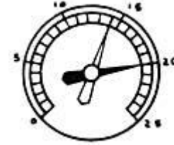
No. 16. If normal is 20 inches and needle should go to approx 14 check timing. Spark may be retarded.
